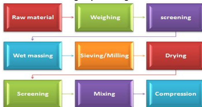
Figure: 2 Wet Granulation Processing Steps
